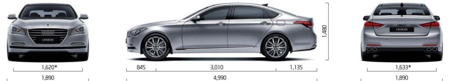
\* Wheel tread • 17" alloy wheels (front/rear): 1,638/1,669 • 18" alloy wheels (front/rear): 1,628/1,659 • 19" alloy wheels (front/rear): 1,620/1,633
